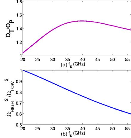
Fig. 3. Plot of (a)  $\frac{Q_T}{Q_p}$  for  $\frac{Q_p}{Q_s} = 1.4$  and (b)  $\frac{\Omega_{HIGH}}{\Omega_{LOW}}$  vs.  $f_s$
