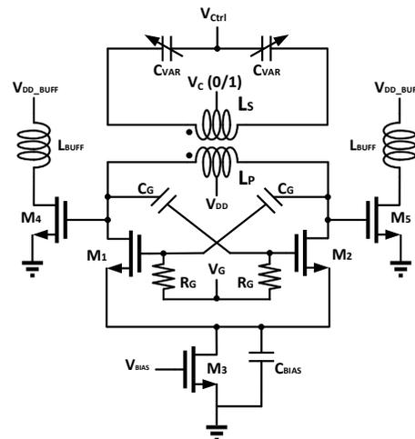
Fig. 1. A Class-C VCO with transformer enhanced tuning range and tank  $Q$
