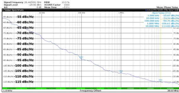
Fig. 7. Measured phase noise at 26.45 GHz
