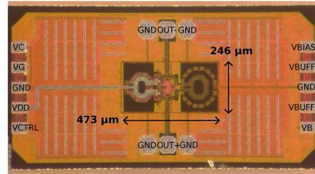
Fig. 5. Chip micrograph of VCO showing core area of  $246 \times 473 \mu\text{m}^2$
