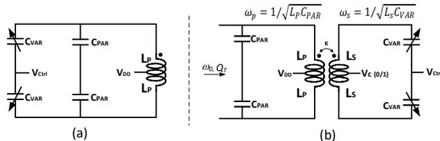
Fig. 2. (a) Conventional LC resonator, and (b) Transformer-enhanced resonator
